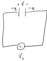
Capacibors are two conductors separated by an insulator. It does not allow DC current to flow, but can
