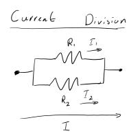
$$I_{1} = \overline{I} \cdot \frac{R_{2}}{R_{1} + R_{2}}$$
