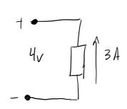
The element delivers power. The Glows Stom a low voltage to a higher voltage.
